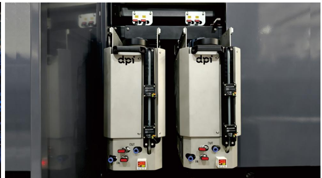
*Constant-Temperature Ink Tank with Agitation System
