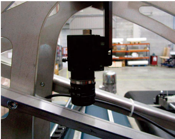
The Cretavision 2.0 compact camera in place
