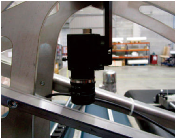
The Cretavision 2.0 compact camera in place
